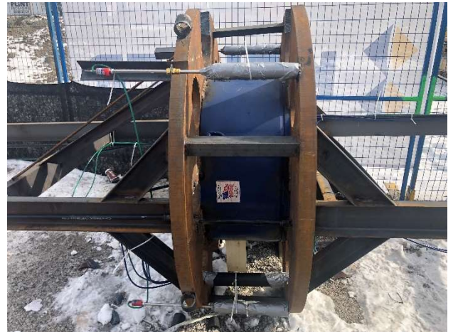
Figure 3. Load cell showing top and bottom plates, LVDTs and other instrumentation.
