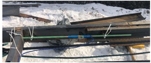
Figure 2. Typical strain gauge rebar setup on the load frame in preparation for a BDSLT.
